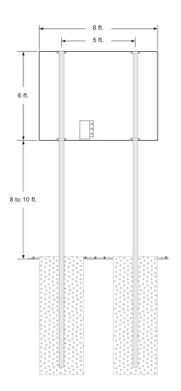
Once you have verified the positions of the posts and the size of the footings, you are ready to dig your holes, pour your concrete, and set your posts. There are several techniques for ensuring proper alignment of the posts. Typically installers will construct a temporary wooden support frame to hold each post in place while the concrete sets. Having plumb posts in the proper position is the key to a smooth mechanical installation.
